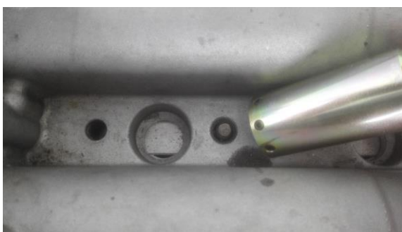
Picture 17: Thread cutting made by ratchet with 19mm socket
