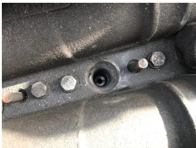
Picture 13: sealing plugs for blind of injector nozzle chamber order item nr. 5055
