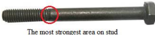
Picture 5. Injector holder stud Fiat Ducato HPi 3.0l
