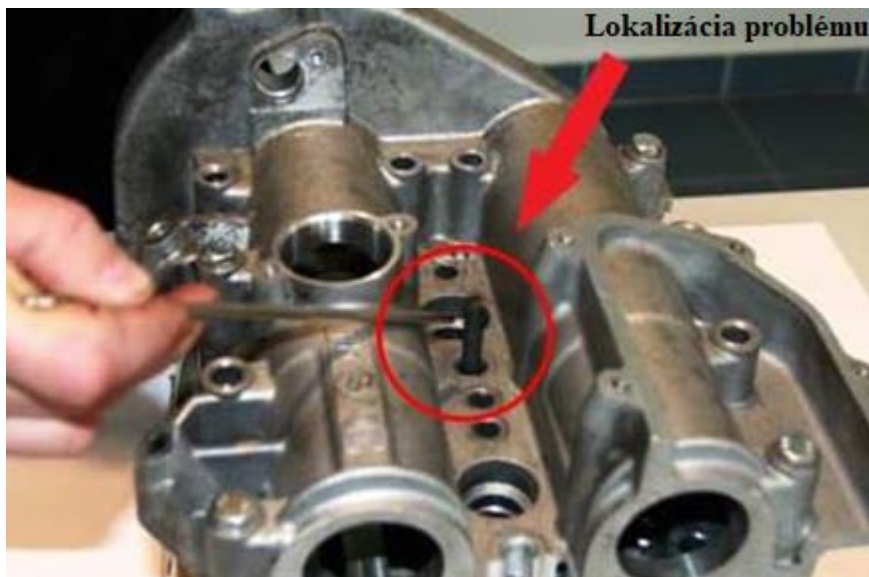
Picture 3. Cylinder head cross section Fiat Ducato HPi 3.0l
