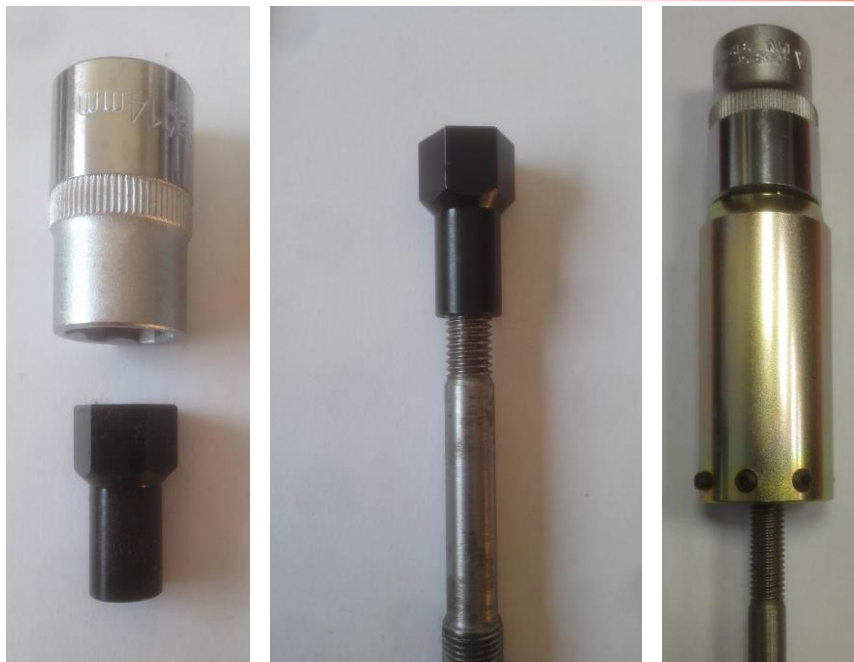
Picture 20: Mounting of a hexagonal nut on the injector older stud.
