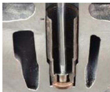
Picture 12: removed injectors, detail of broken stud without other changes
