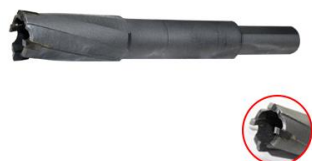
Picture 7. When stud is broken under the engine cover is need to drill broken stud by hollow cutter item nr 10140.
