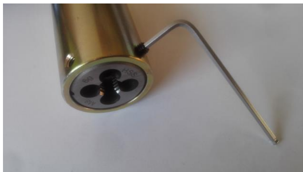
Picture 16: installing of threaded die into the die holder using by 2mm allen key
