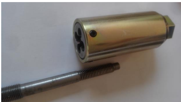
Picture 18: Cutting of sufficient thread numbers for protruding part broken stud M8.
