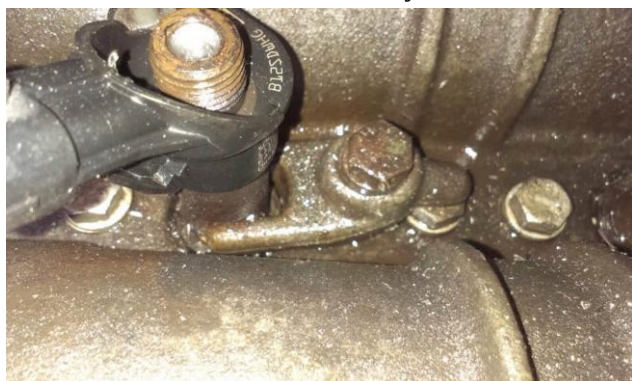
Picture 10: problem localization: installed injector, holding by injector holder and fixing bolt.
