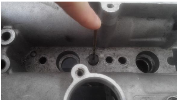
Picture 11. Instruction for drilling of hexagon head of holder 's stud of injector – using of center punch and drill 3mm Fiat Ducato HPi 3.0l
