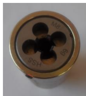
Picture 16: installing of threaded die into the die holder using by 2mm allen key
