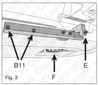
6. The bush (**F** in Figure 3) can now be extracted. Lubricate the force screw (**B15**) with molybdenum disulphide grease, then assemble the puller as shown in Figure 4. Holding the anti roll bar up 0to gain clearance, place the bush collar (**B4**) up over the subframe and onto the bush; secure onto the force screw (**B15**) with the top nut (**B12**).
